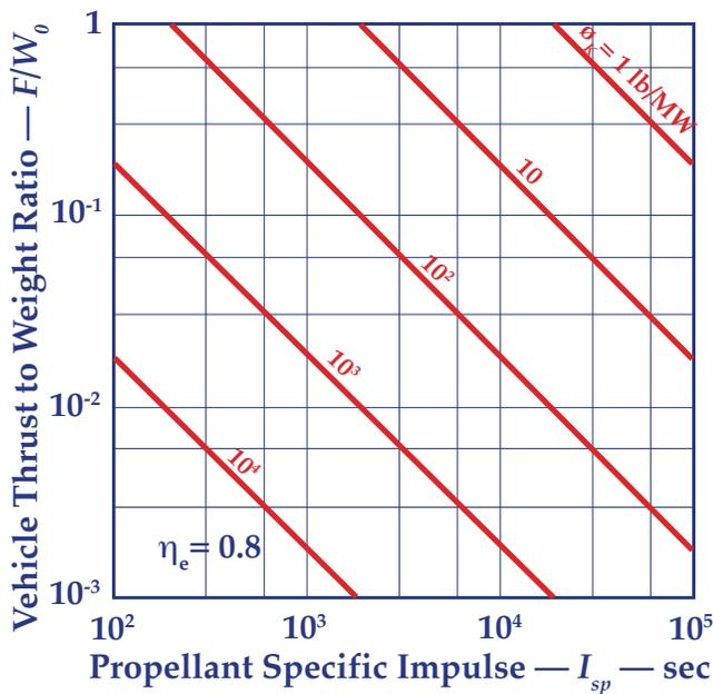
Figure 5 — Generalized Performance of Reactor System Powered Vehicles
