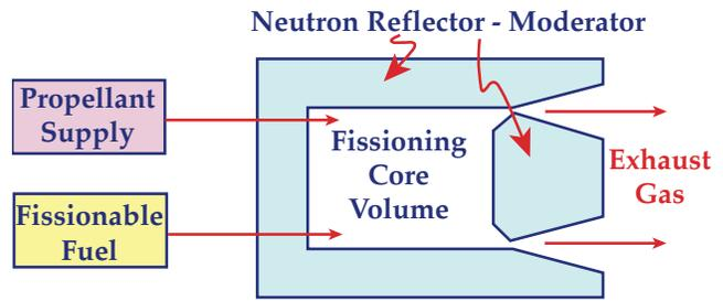
Figure 1 – Gaseous "Cavity" Reactors
