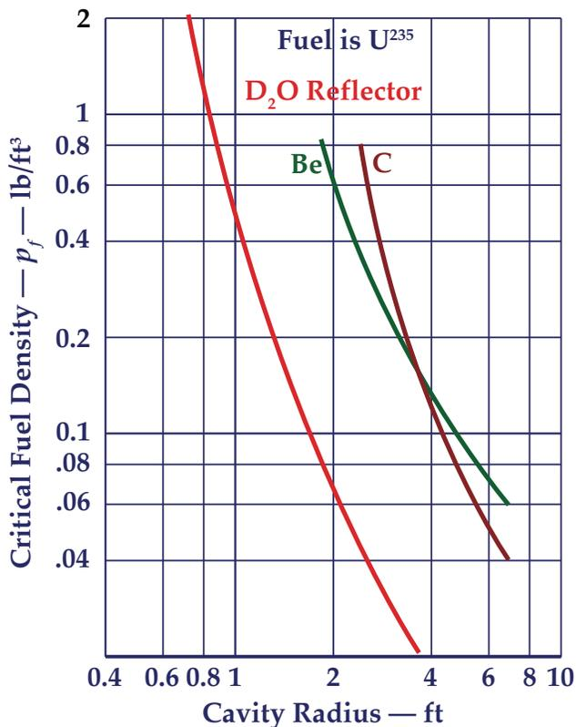
Figure 2 — Critical Fuel Density in “Cavity” Reactors
