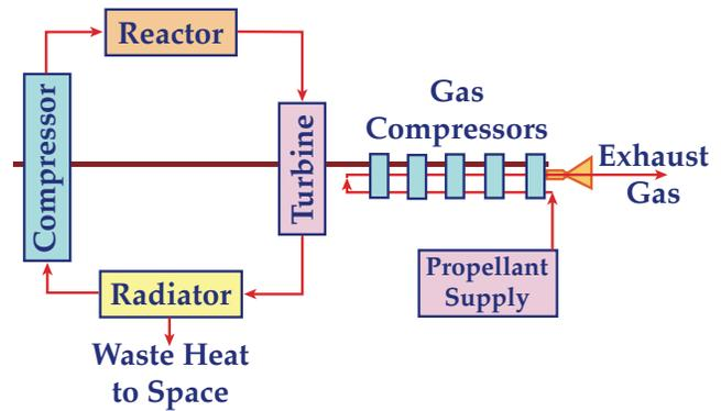
Figure 3 — Thermo-mechanical Gas Compression Systems
