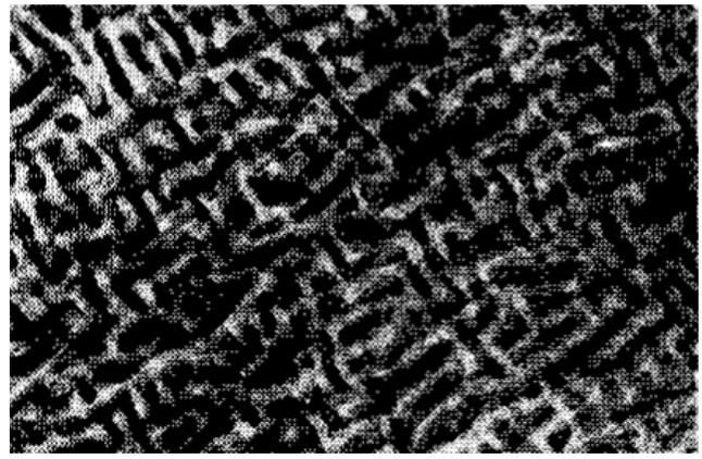
Figure 1e — Magnet microstructures resulting from spinodal decomposition. Cunife transmission micrographs (P. Tufton, thesis, University of Cambridge, 1963). Magnification marker corresponds to  $0.1 \mu$
