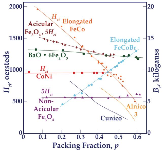
Figure 2 — Effect of packing of magnetic phase on intrinsic coercive force for materials with predominantly crystal anisotropy BaO 6Fe20a, CoNi, and non acicular FeaO, particles; and with predominantly shape anisotropy-elongated FeCo particles and a series of Alnico 3 and Cunico alloys. Acicular FeaO particles show contributions from both shape and crystal anisotropy.
