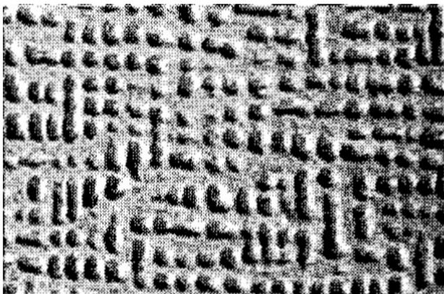
Figure 1d — Magnet microstructures resulting from spinodal decomposition. Alnico 8 replica perpendicular to the field-treating direction. Reference same as 1a.
