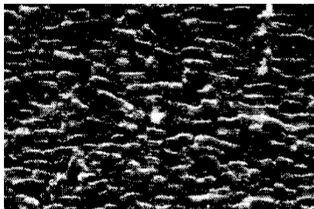
Figure 1a — Magnet microstructures resulting from spinodal decomposition. Alnico 5 micrograph of replica parallel to field treating direction, J. de Jong, J. Smeets, and H. Haanstra; *Journal of Applied Physics* 29, pp. 297 (1958)
