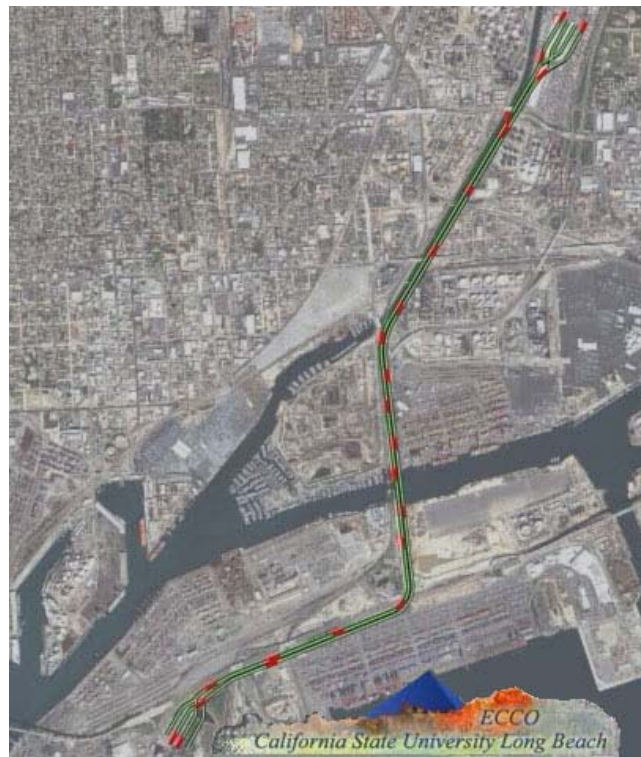
Figure 7 Alignment for Port of LA/ECCO Project
