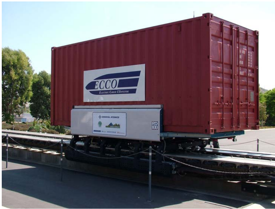
Figure 3. World's First Maglev Container Move at General Atomics San Diego, CA, June 2006.
