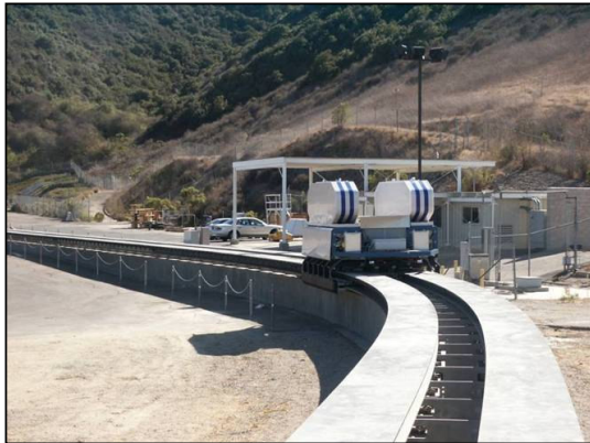
Figure 8. Testing the chassis with water tanks installed.
