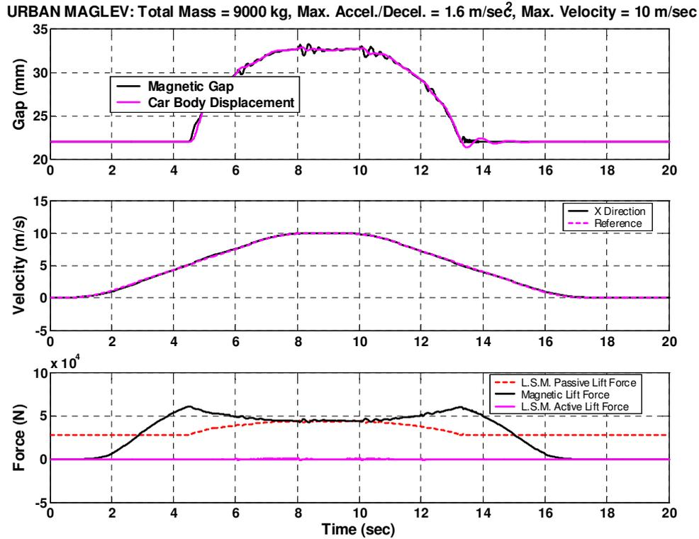
Figure 6. Simulation of Missing Position Location Pulses Every 2 seconds. Error Size: 20mm, offset duration: 50 ms,  $V_{max}$ : 10 m/s,  $accel_{max}$ : 1.6 m/s<sup>2</sup>, mass: 9000 kg
