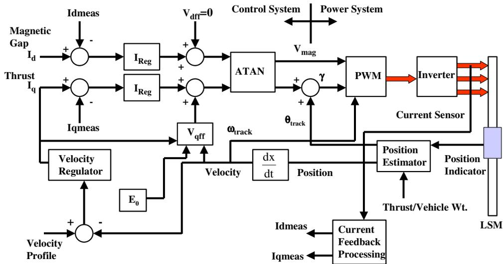
Figure 7. UML Control System Schematic
