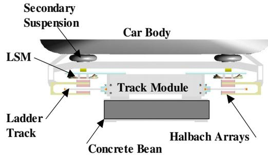
Figure 2. Vehicle-to-Guideway Arrangement
