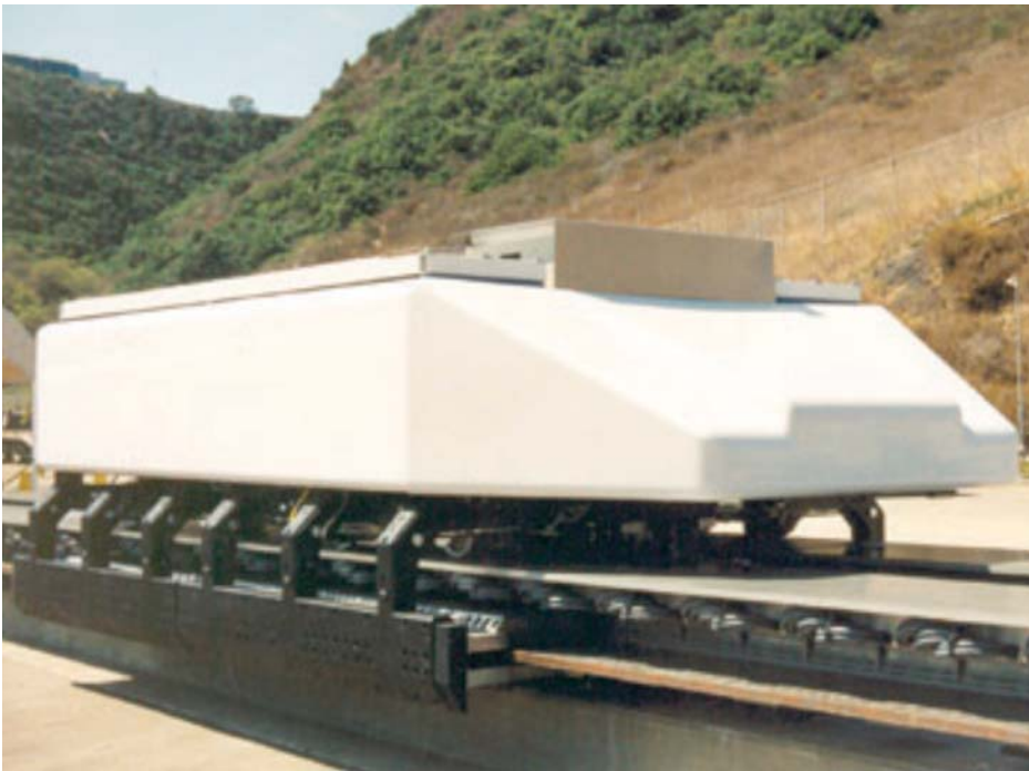
General Atomics' full-scale Inductrack test vehicle on the first section of the test track.
