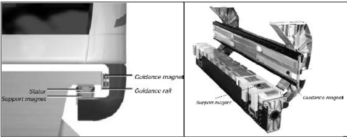
A diagram showing one of the J-shaped extensions of a Transrapid train wrapping around its guideway. The support magnet levitates the train and the guidance magnet keeps the train centered on its track. On the guideway, the stator produces alternating electromagnetic waves that propel the train forward.
