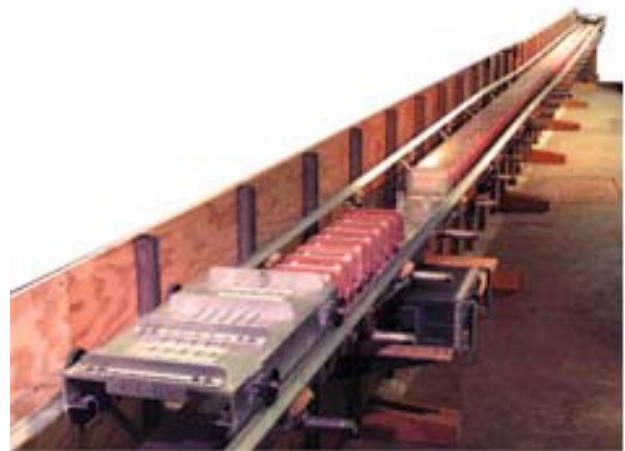
The 20-meter test track at Lawrence Livermore Laboratory used drive coils in its first 4.5 meters for propelling a 20-kg cart to 20 m/s. That was about six times the speed needed to levitate the vehicle.
