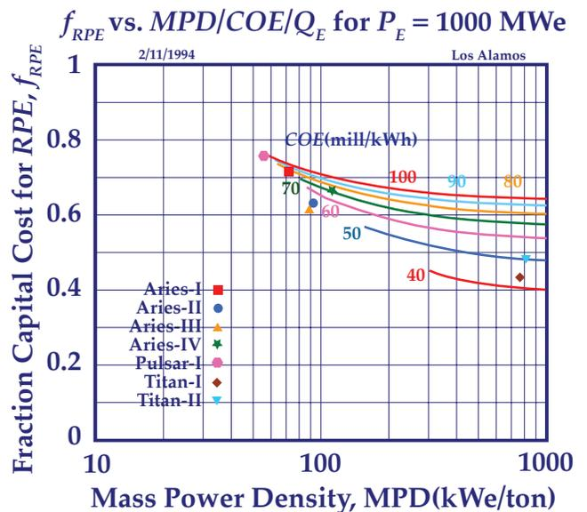
Figure 6 — Parametric dependence of fraction of *TDC* (including contingencies) allocated to the *RPE* (Account 22.1, Table 1) on *FPC MPD* for a range of *COE* values for a  $P_E = 1000$  - MW(electric)(net) fusion power plant described by the parameters listed in Table 2. Optimized design points from a number of recent tokamak<sup>4-6</sup> and *RFP* (Reference 14) reactor studies are also shown. The design points for ARIES and TITAN generally reside at or near the top of the
