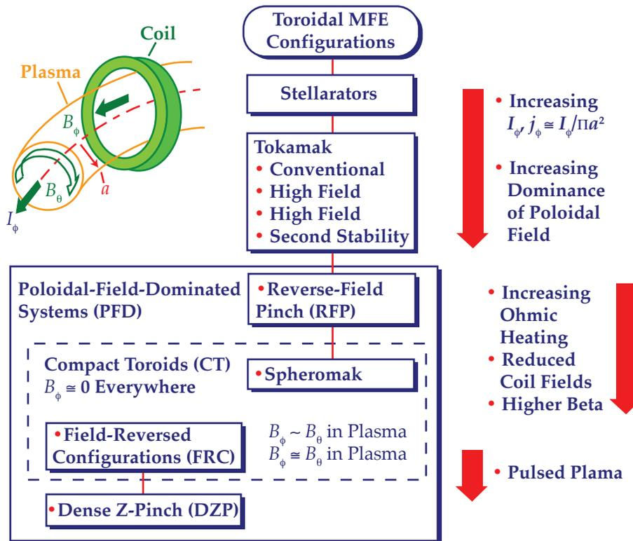
Figure 9 — Spectrum of main *MFE* configurations ordered according to toroidal (axial) current density and domination of poloidal magnetic field; starting with SSR and spherical torus tokamaks. a lineage of *MFE* concepts is identified that reduces reliance on externally applied magnetic fields and the economic and operational problems such fields create for the *MFE* power plant extrapolation.<sup>4-7,25,30</sup>
