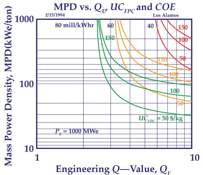
Figure 8 — Parametric dependence of  $FPC$   $MPD$  on engineering gain for three  $COE$  values and three  $FPC$  (composite) unit costs for the fusion power plant described by the parameters listed in Table 2.
