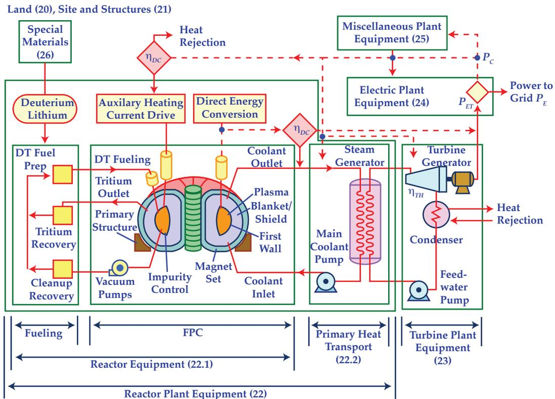
Figure 1 — Fusion power plant layout showing essential systems functionally organized into major cost-account blocks (Table 1).
