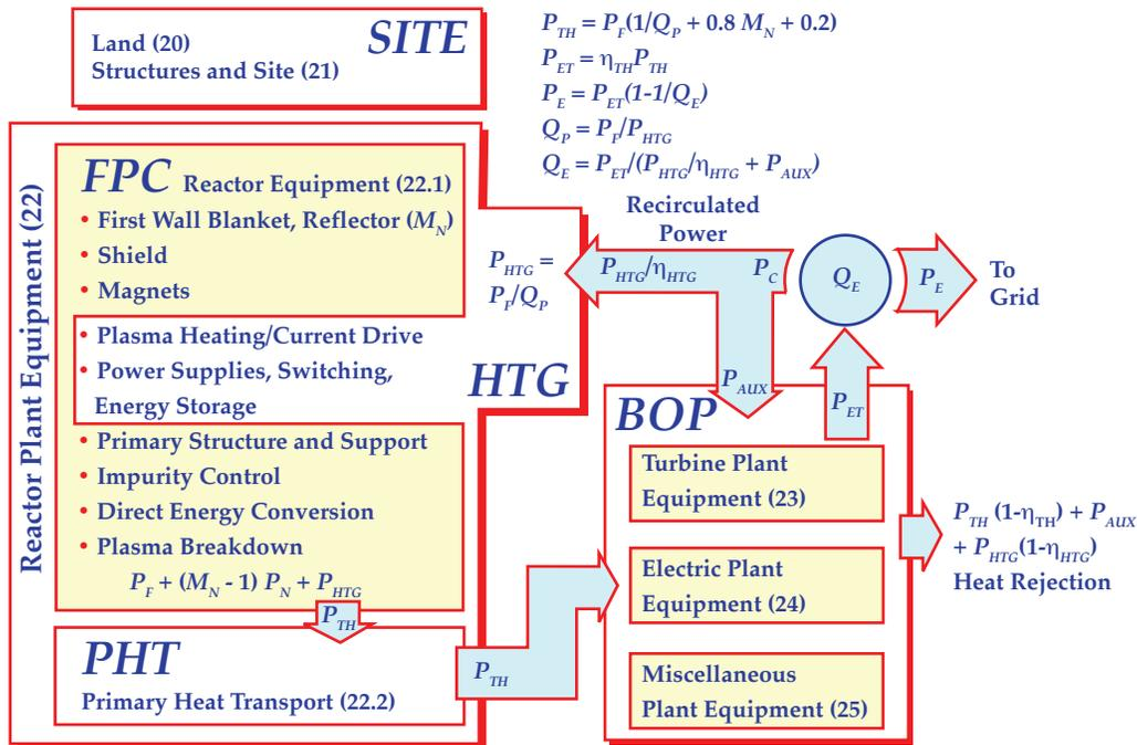
Figure 3 — Condensed fusion power plant costing model and associated power flows (Table 1).
