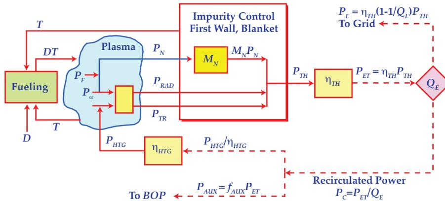
Figure 2 — Simplified energy flows used to model fusion power plant cost.
