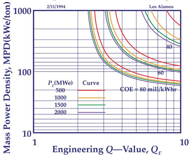
Figure 7 — Parametric dependence of  $FPC$   $MPD$  on engineering gain for a range of  $COE$  and  $P_E$  values for the fusion power plant described by the parameters listed in Table 2.
