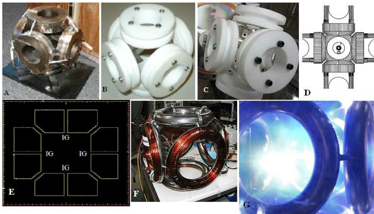
Figure: Different polywell reactors, built, planned or simulated. A) WB-3 developed by Dr. Bussards' team from 1998 to 2001. This device had a radius of 10 cm or 4 inches [23]. B) A picture of Dr. Khachans' device developed at the University of Sydney, Australia, in 2009 [6]. This device had a width of 6 cm or 2.3 inches. C) A picture of Mark Suppes device built in Brooklyn New York, in 2011 [24]. D) A schematic of a reactor, patented by Joel Rogers, November 10 th 2010. A modification on the polywell design, indications are that this will be over 2 feet a side [4] E) A figure of the polywell design simulated by Iranian researchers in October 2011; this was over two feet to a side [5]. F) A picture of WB-6 developed by Dr. Bussards team in the summer of 2005; this device was about 1 foot a side [23]. G) A picture of WB-8 being operated in 2008 [23].
