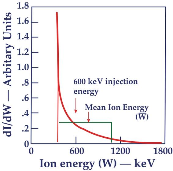
Figure 3 — The expected energy distribution<sup>5</sup> compared to the flat-topped distribution used in the report.
