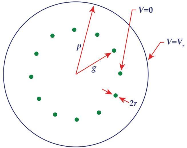
Figure 10 — Simplified geometry for calculating the electric field at the grid wires.
