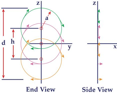
Figure 4 — Nine trajectories used at each energy to define the incident beam at the magnetic mirror. Larmor radius ( $a$ ) depends on energy.
