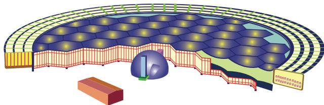
Figure 1 — A mirror-type reactor surrounded by the magnetic expander and direct recovery system.
