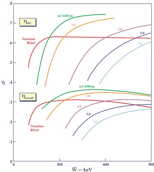
Figure 14 — Working efficiency ( $\eta_{DC}$ ) of the direct converter, and overall plant efficiency ( $\eta_{overall}$ ) versus mean energy. The curves labeled Venetian Blind refer to a direct converter.
