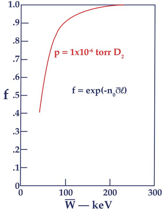
Figure 12 — The fraction of the  $D^+$  ions that do not charge exchange vs mean ion energy. Pumping speed and beam power are held constant.
