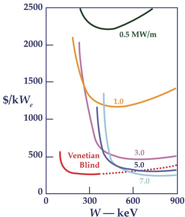
Figure 16 — Cost estimate for the direct converter per net kW out of the reactor as a function of mean ion energy.
