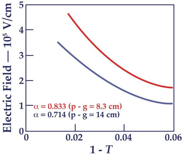
Figure 11 — Electric field at a grid wire vs the optical opacity of the grid. (See Figure 10 for p-g.)
