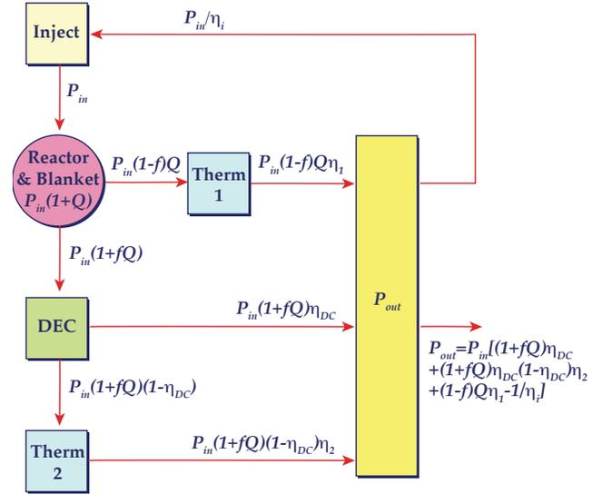
Figure 15 — Power flow diagram for a mirror reactor with a direct converter.
