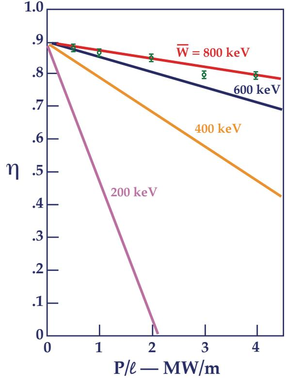
Figure 5 — Collection efficiency versus power level for several different mean energies.
