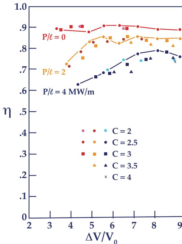
Figure 8 — Collection efficiency versus potential difference between an opposing pair of focus electrodes across the channel from each other.
