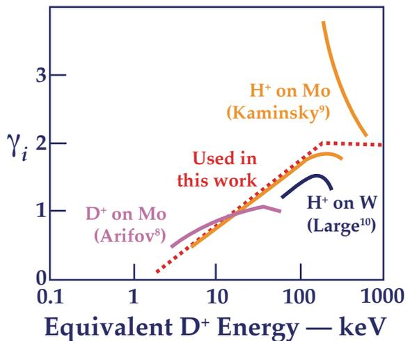
Figure 9 — Secondary electron emission coefficient vs ion energy.
