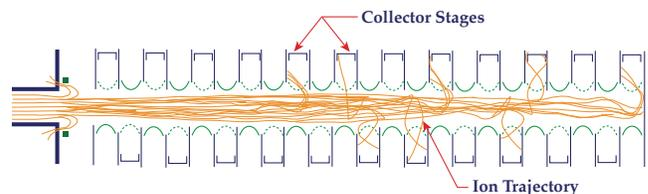
Figure 2 — Ion trajectories inside the focusing and collecting system.
