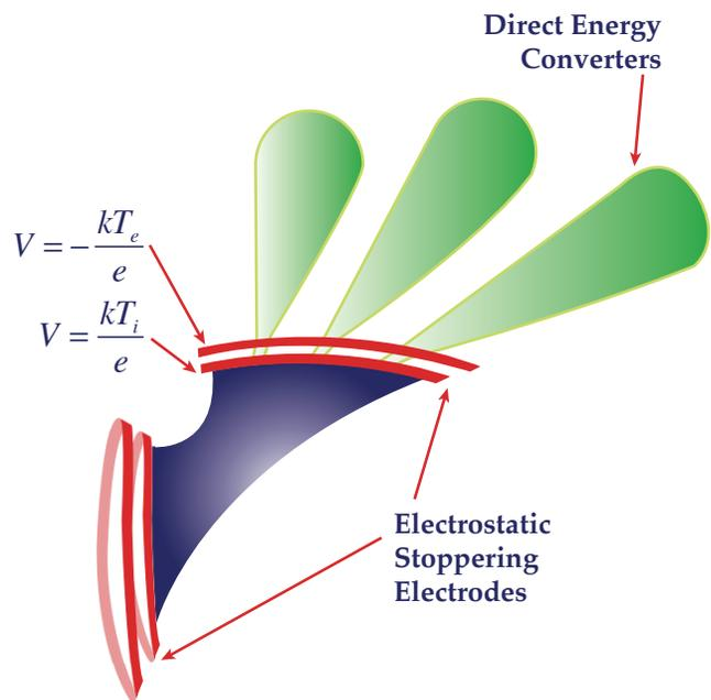
Figure 13 — Venetian Blind direct energy converter. The figure shows how electrostatic stoppering might be used to make the leakage of plasma from the mirror reactor more selective.
