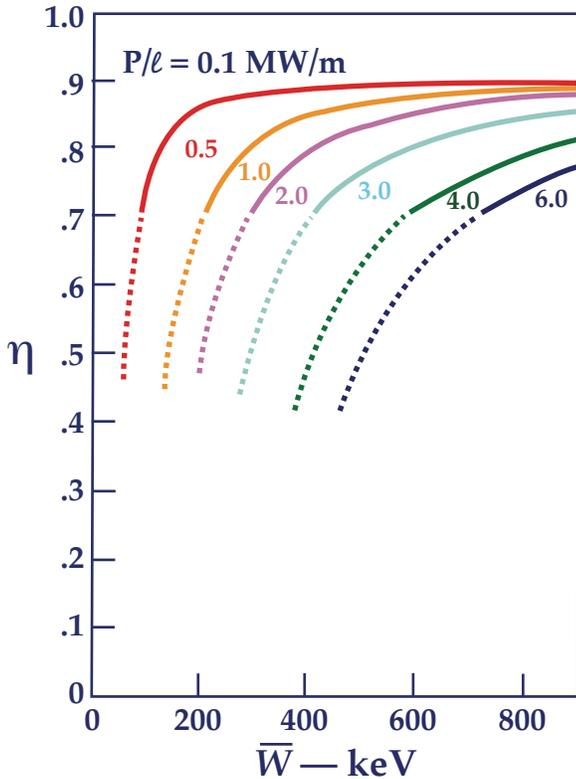
Figure 6 — Collection efficiency vs mean energy for different power levels.
