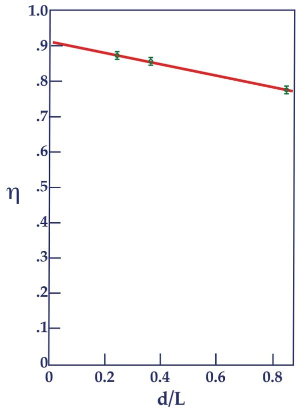
Figure 7 — Collection efficiency vs beam thickness ( $d$ ).
