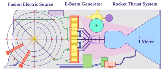
Figure 1 – Schematic outline of ARC/QED engine system
