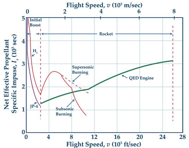
Figure 7 — Net  $I_{sp}$  vs. flight speed; SSTO system
