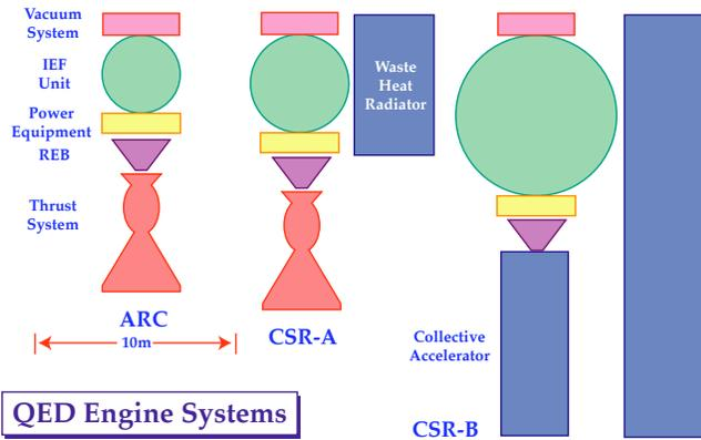
Figure 2 — Schematic outline of sequence of QED engines
