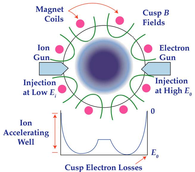
Figure 4 — The EXL/IEF concept; ion acceleration by electron-injection-driven negative potential well maintained in polyhedral magnetic field
