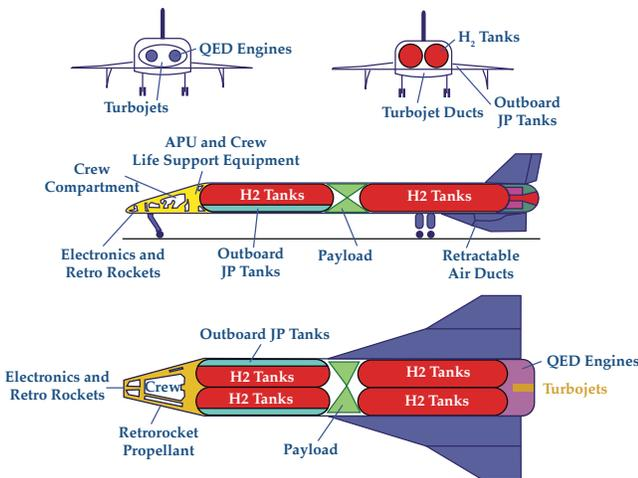
Figure 6 — Schematic outline; QED/ARC SSTO vehicle
