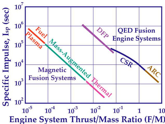
Figure 3 — QED engine performance, showing  $I_{sp}$  variation with thrust-to-engine-mass ratio  $[F]$  compared with conventional magnetic fusion concepts.<sup>5</sup>
