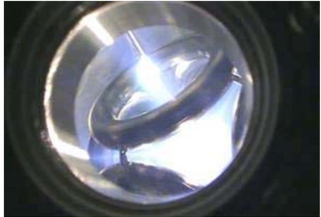
A test plasma using helium glows inside the WB-7.
